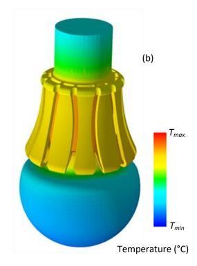
Figure 2: The new LED replacement light bulb (a) and surface temperature plot in 6Sigma (b).
